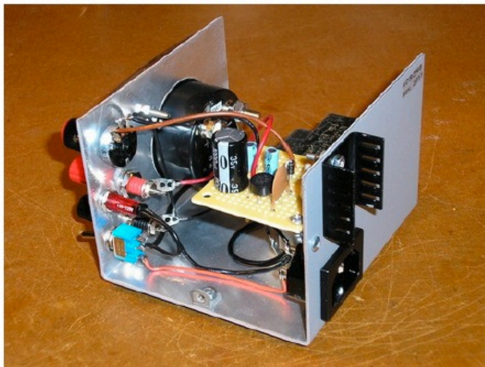
Figure 4. The interior of the completed unit. The circuit board is mounted on the enclosure's back wall so that the LM317T can be in thermal contact with the enclosure.
