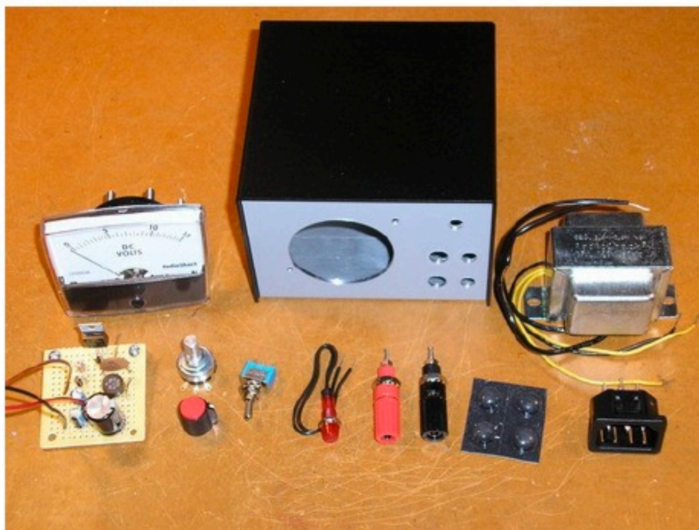
Figure 2. The parts of the supply, ready for assembly. The circuit board that holds the rectifier, filter, and regulator is at the lower left.
