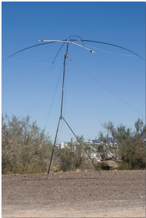
A homebuilt "Moxon" HF antenna
